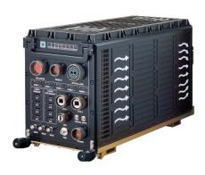
SPAS is the most versatile sonobuoy processor system for ASW platforms. SPAS makes use of advanced proprietary processing technologies for adding automation to the detection and classification of submarine threats, which reduces the operator's workload
