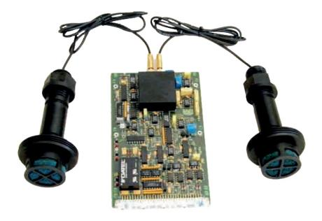
SAES has designed and developed the SET-200/P to measure the Underwater Electric Field at sea. SAES UEP sensor is a precise, ultra-low noise device that enables measurement of low-level electric fields.
